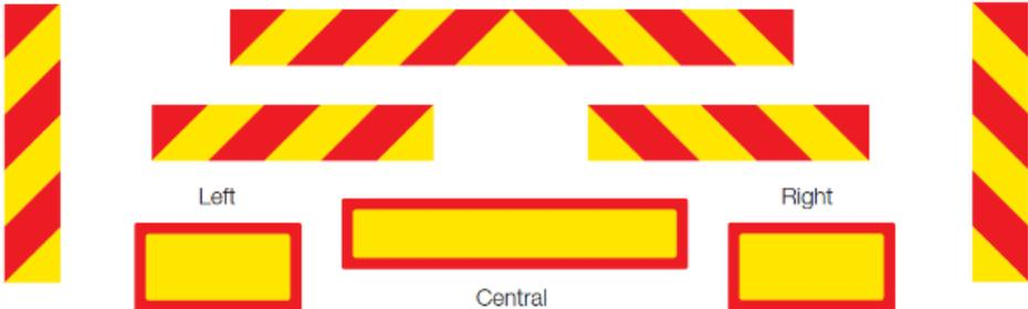
Such marking must be fully reflective vehicle signs, conforming to B.S. AU152.
