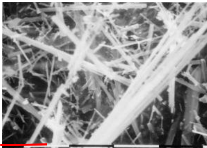
Figure 1- amosite ( Brown asbestos) under SEM.
