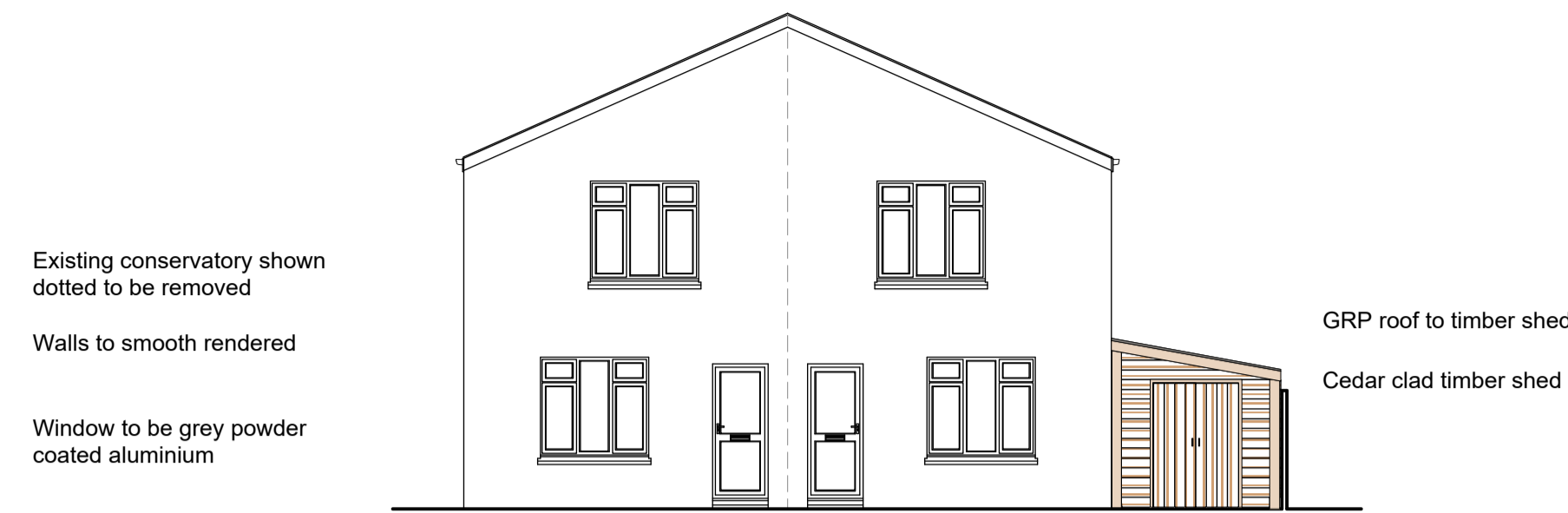
SOUTH WEST ELEVATION
