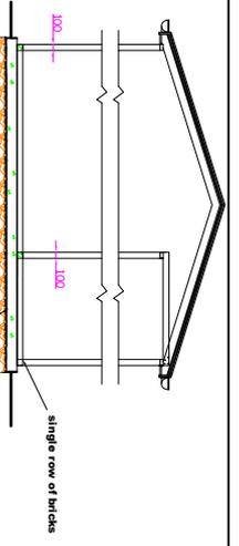
well consolidated hardcore with stone dust bedding over then 150mm concrete slab. Ensure details are supplied by the stable manufacturer. Each unit differs and the setting out of the slab is very important.
