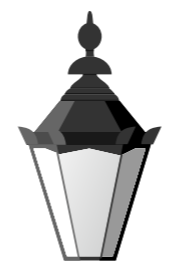
Sign F - 1:20 One black Stratford lantern Sizes 380 x 660mm, G/Cl - 2600mm, D - 600mm.
