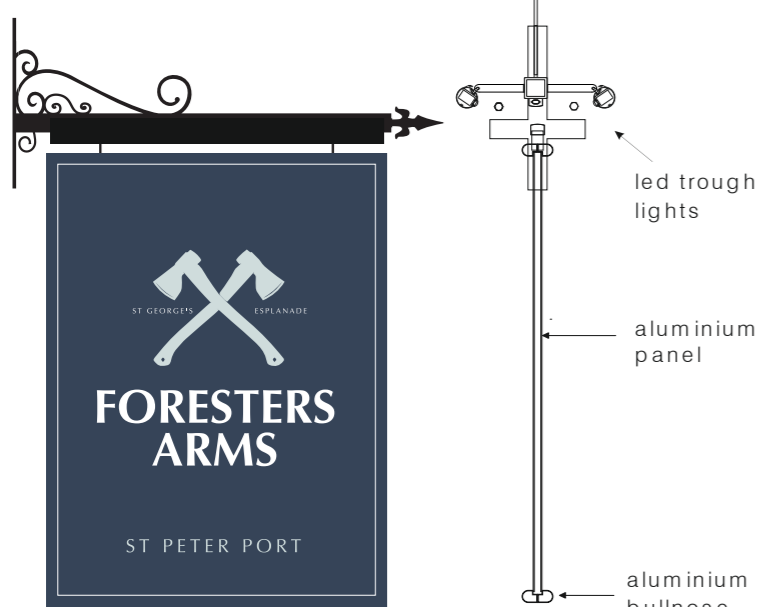
Sign B - 1:20 One aluminium bullnose projecting signs complete with steel gibbet Illuminated by led trough lights. Sizes 900 x 1200mm, G/Cl - 3980mm, D - 80mm.
