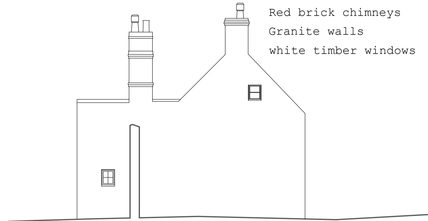
West Elevation 1:100 (Main house)
