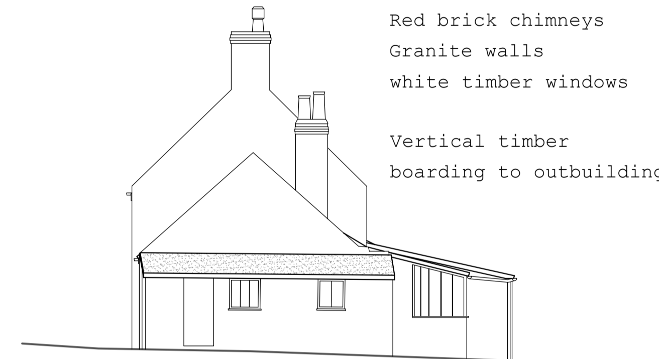
East Elevation 1:100 (Main house)
