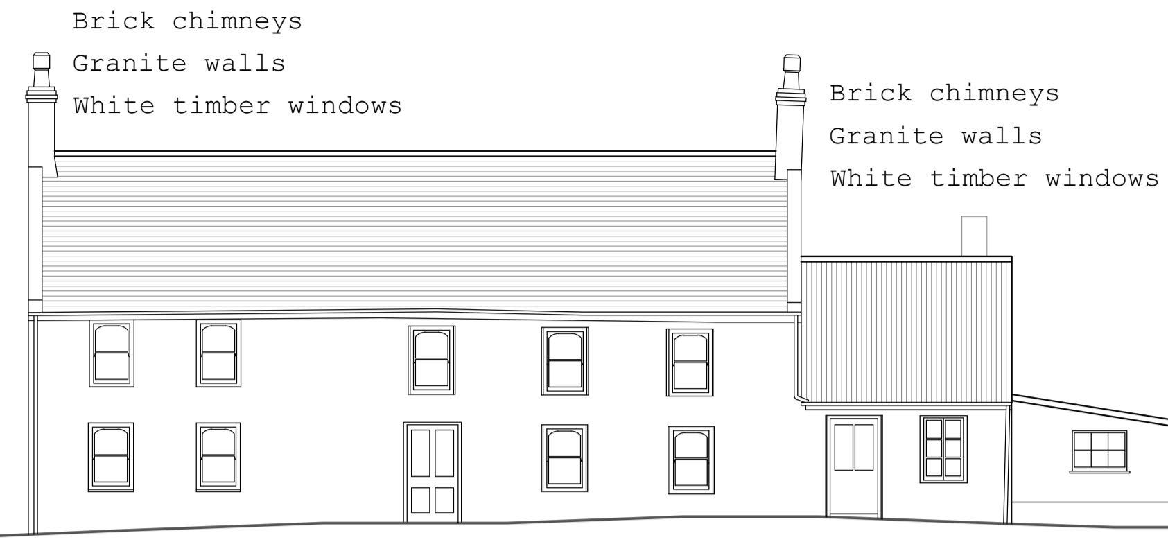
South Elevation 1:100 (Main house)
