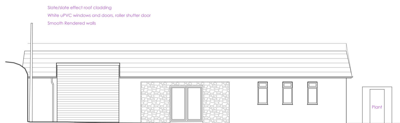
Existing South Elevation 1:100
