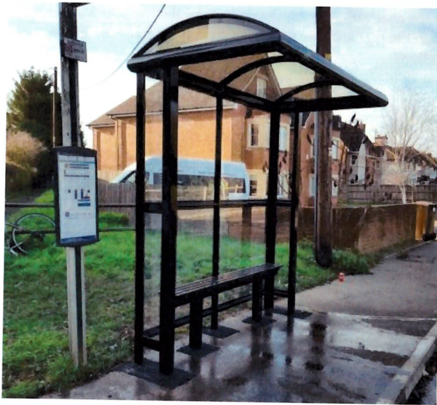
Figure 2 Illustrative All-Weather Cantilever Shelter (two bay).
