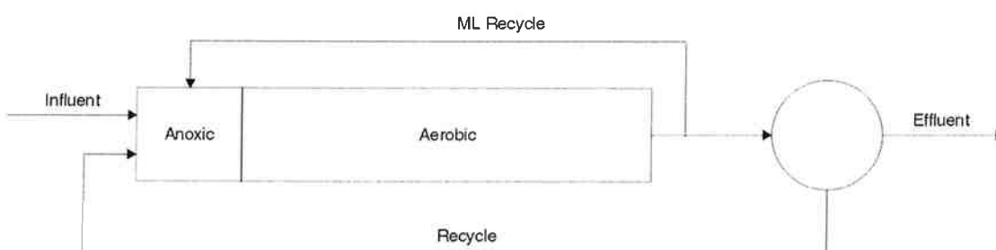
Figure 4.2 Activated Sludge Process with Mixed Liquor Recycle
