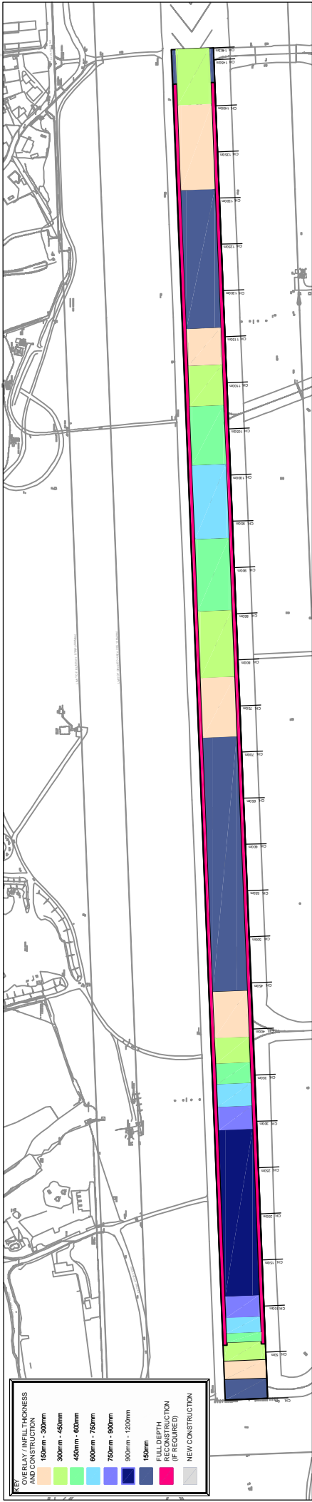
RUNWAY PLAN ILLUSTRATION OVERLAY AND INFILL THICKNESS TO ACHIEVE PCN OF 36
