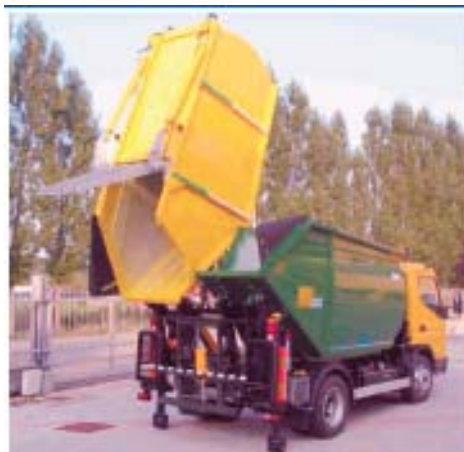
Figure 3: Rear loading dual compartment RCV (Ecofar)
